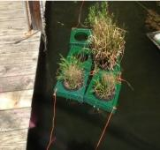
Here's a sneak peek at two new PVC based designs currently undergoing float testing in the Magothy River.
